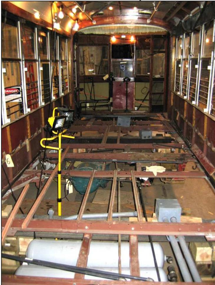
*Interior of Car 25 showing new piping and air tanks, compressor and brake cylinder in place, and electrical conduits partially installed.*
