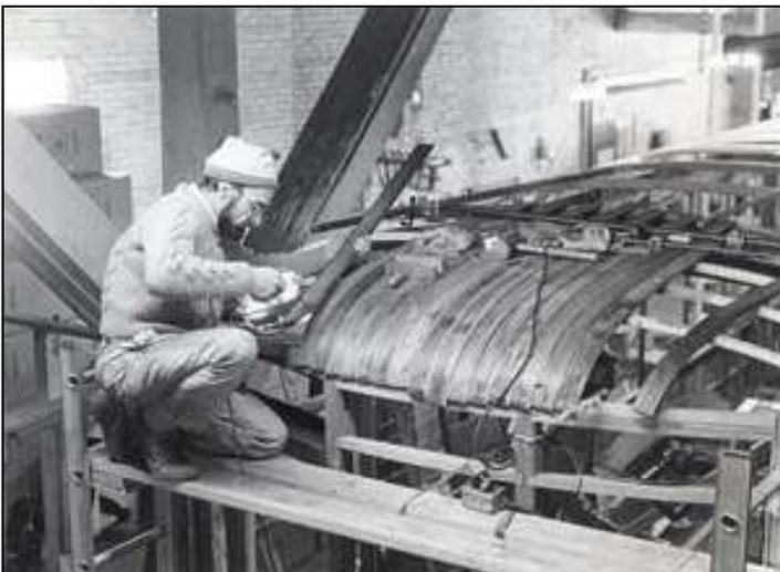
*Roger Smith custom-bent new roof boards on Car 21 in the Howes barn in the early 1980s. Three decades later, he has completed six new cherry sashes for Car 25's end windows and rebuilt most of the side sashes. Bob Browning has finished and installed new laminated safety glass in the end windows and is now refinishing the old doors.*
